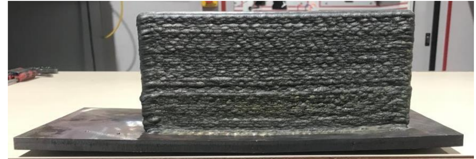
Figure 3: Wire-DED fabricated part & Distortion accumulation can lead to rejection of part
