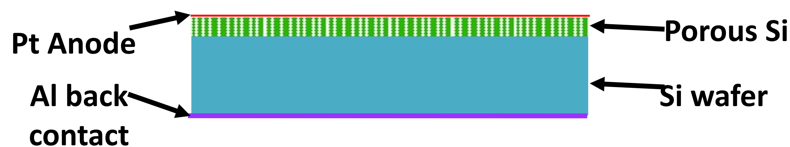
Figure 1. Schematic of fuel cell device
