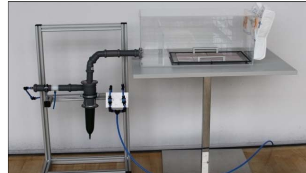
CAD rendering of the artificial dusting device
