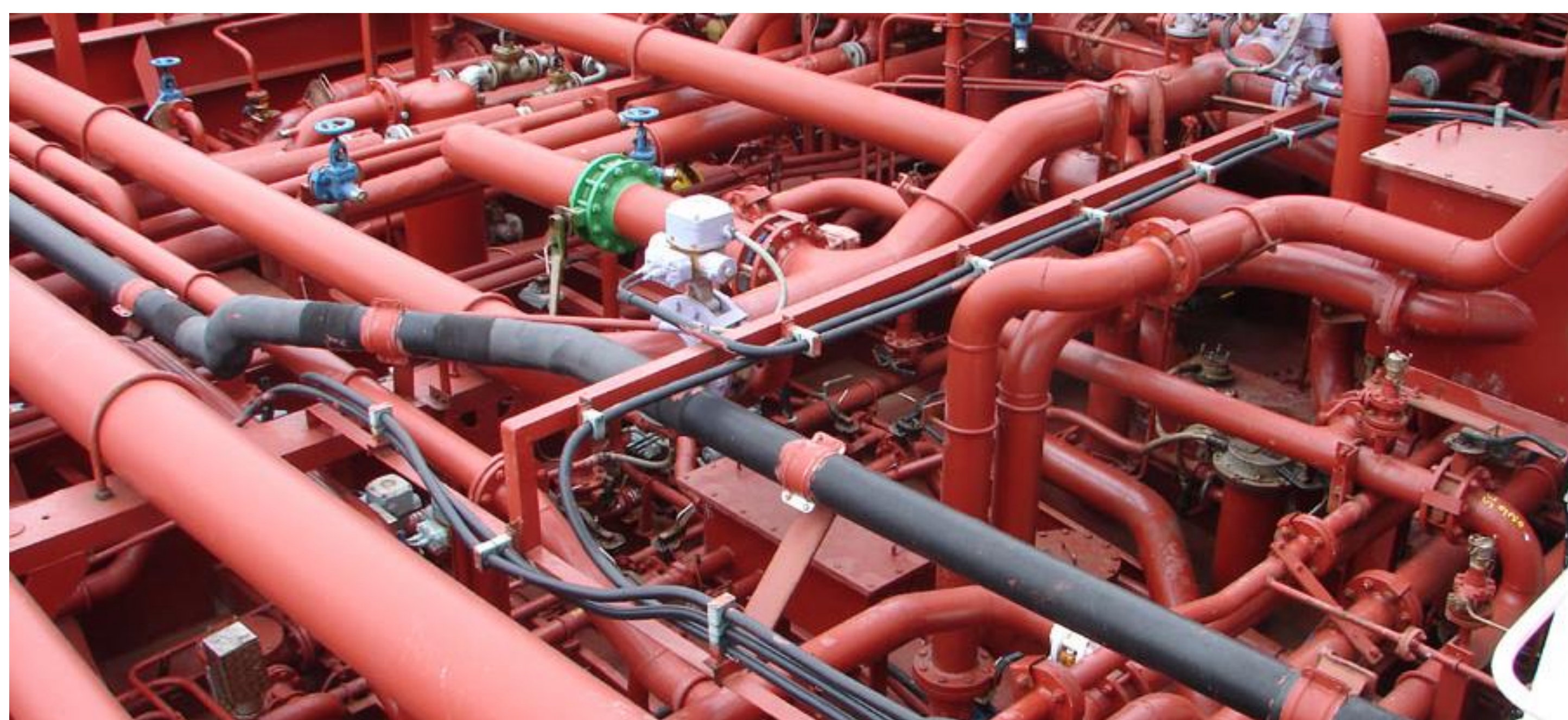
FIGURE 1. Piping systems on an oil/chemical tanker. Image licensed under CC BY-SA 3.0 via Wikimedia Commons.
