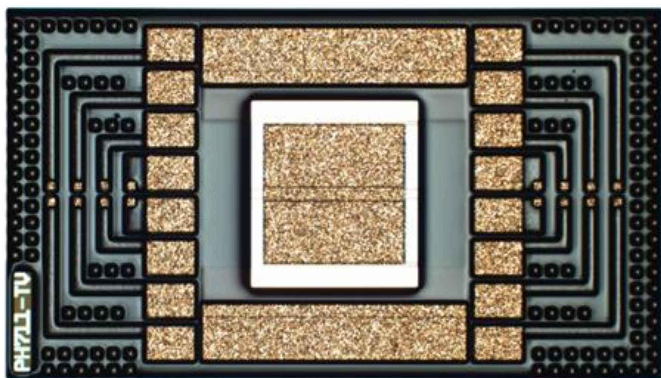
Fig. 1 Light microscopy image of a test device showing copper pads for electrical functionality and central copper square subjected to thermomechanical loading.
