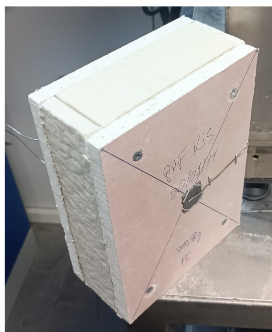
FIGURE 1. Left: Small-scale test piece for insulation testing, consisting of plasterboard mounted on both sides of a metal stud and insulation in the center. Right: Temperature measurements and results from the app.
