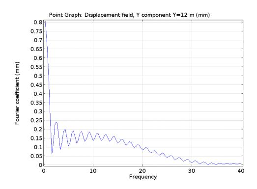
With barrier, applied force of F=1000 [kN] at lower boundary, Vp=124,91 [m/s], mesh size= 0.1 [m], time step= 0.001 [m], quadratic triangle, relative tolerance=0.001, fm=45 [Hz]
