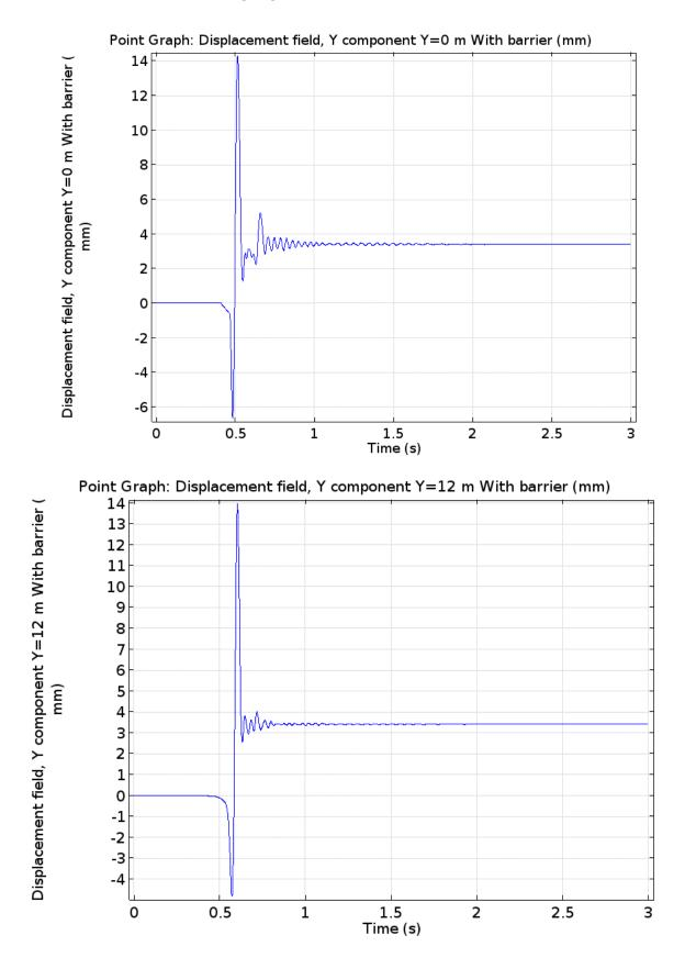
With barrier, applied force of F=1000 [kN] at lower boundary, Vp=124,91 [m/s], mesh size= 0.1 [m], time step= 0.001 [m], quadratic triangle, relative tolerance=0.001, fm=45Hz
