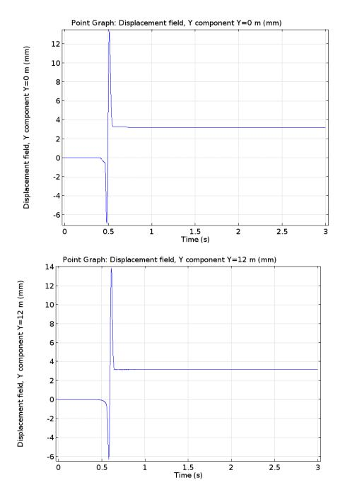
Without barrier, applied force of F=1000 [kN] at lower boundary, Vp=124,91 [m/s], mesh size= 0.1 [m], time step= 0.001 [m], quadratic triangle, relative tolerance=0.001, fm=45 [Hz]
