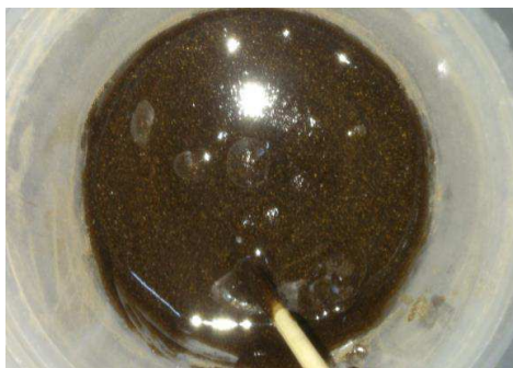
Figure 1: RHCNTs after stir with polyester and MEKP.
