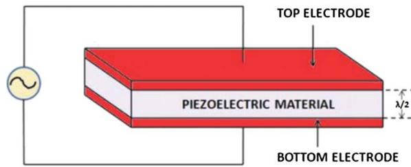
Figure 1: Schematic of TFBAR.
