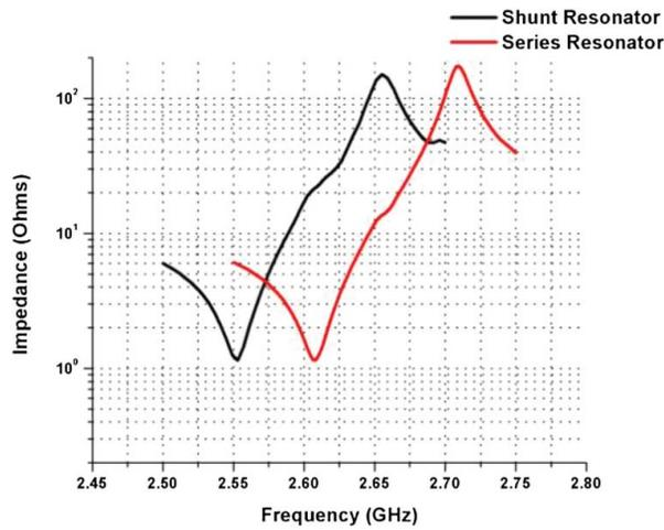
Figure 4: Impedance versus frequency response of the series and shunt resonators.
