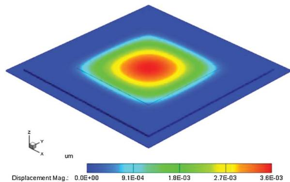
Figure 5: Displacement along  $z$  direction with a 1 V DC.
