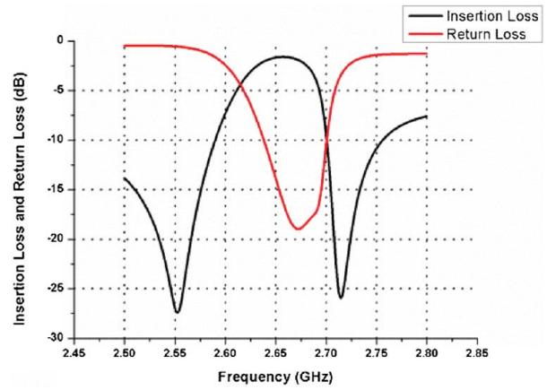
**Figure 8: Response of third-order filter.**
