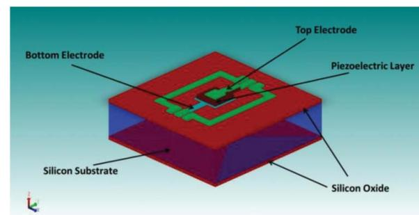
Figure 3: Designed TFBAR structure.
