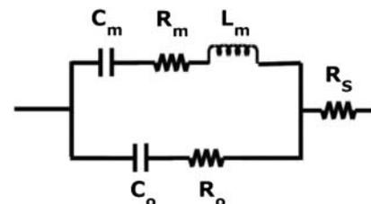
Figure 6: MBVD equivalent model of the TFBAR.
